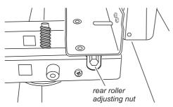
Make 10 complete (360°) turns clockwise. (This means turning and removing the levelling tool 20 times).
